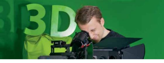
from the main camera. This means that work on set is almost like during a 2D production." Software used during editing takes the images from this camera system and calculates depth maps – images that use various gray tones to show how far the object at a certain pixel is from the viewer. The software uses these depth maps to generate the two camera perspectives needed for the optimum 3D image, whether it's for the screen in a movie theater or for TV.
